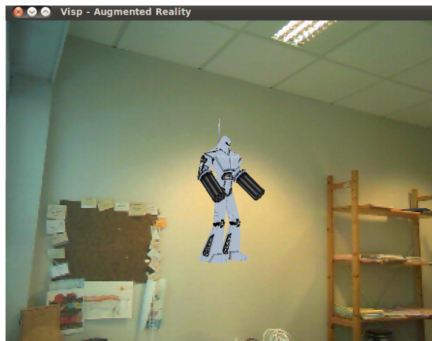
Figure 1: A snapshot of the rendering produced by HelloWorldOgre.cpp . Color images acquired by an available framegrabber are used as a background texture, while a robot is projected in the scene at a static position with translation coordinates (0, 0.05, 0.05) and rotation coordinates (\pi, -\pi/4, 0) .
